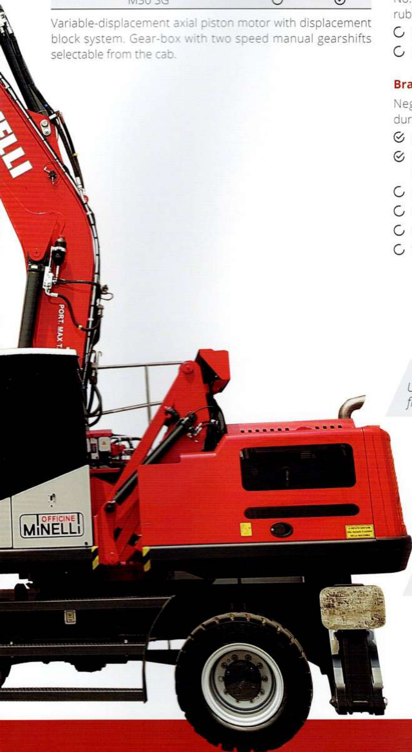
Undercarriage with rear & front outriggers
